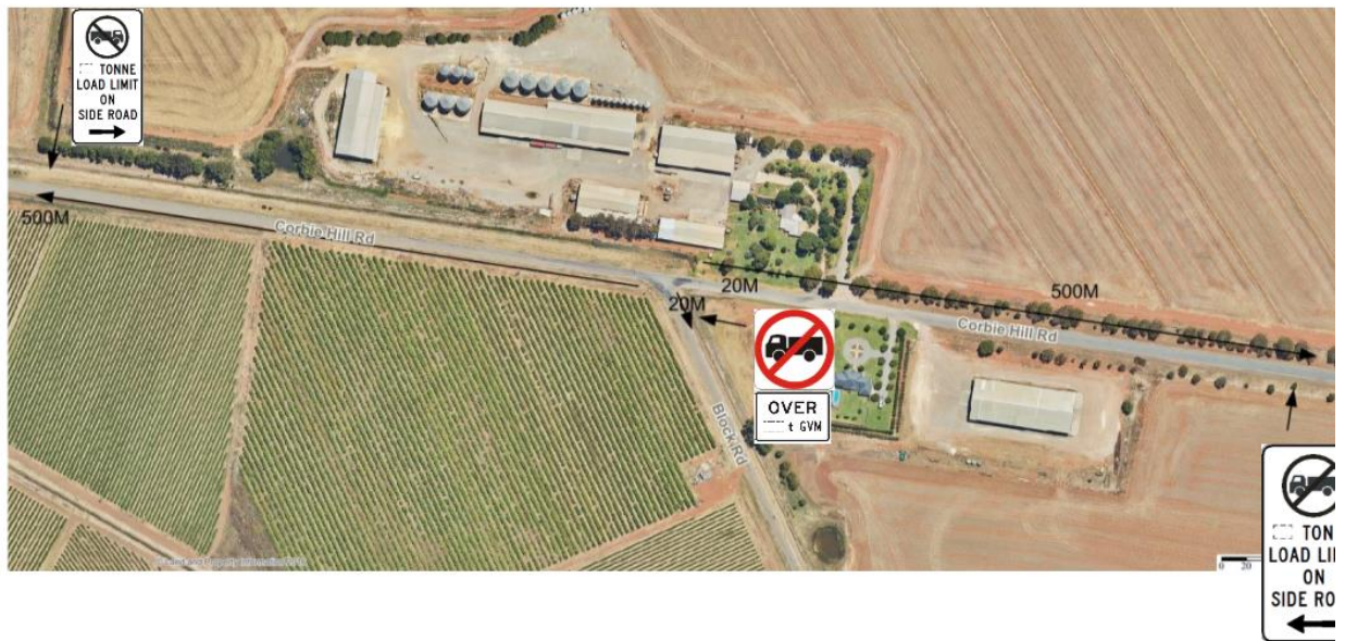
Image 1 above: indicates the proposed 10t limited signage for Block Road and the warning signage for Corbie Hill Road.
