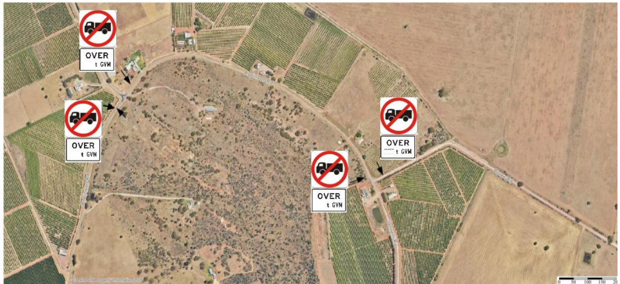
Image 2 Above: Shows where reminder Trucks prohibited and 10t load limited signage will be placed on Robinson Road. They will all be placed 20m after the intersection.
